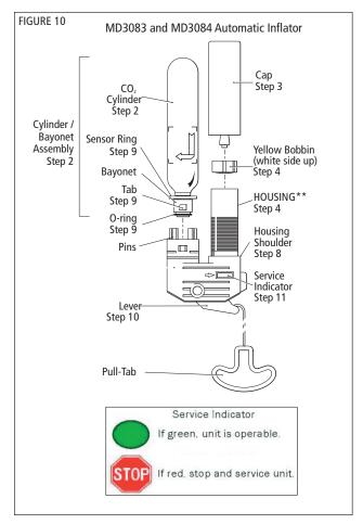
6) Inspect the bobbin. If the bobbin has been fired or damaged, replace it! Ensure the new bobbin is valid, it must have been purchased within the last three (3) years. If the bobbin purchase date is
